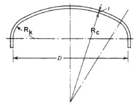
These heads have the crown radius equal to less than the diameter of the head. To reduce the stresses at the corner of the head, a knuckle is formed with a radius of at least 6% of inside diameter. The thickness of such heads is given by:
