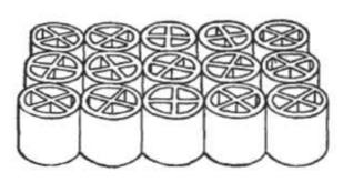
**Stacked packing**: cross-partition rings, packing size: 3/4"
