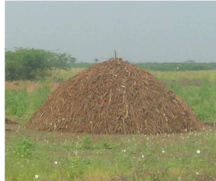
A heap of semai karuvil wood for charcoal production (before covering with soil)
