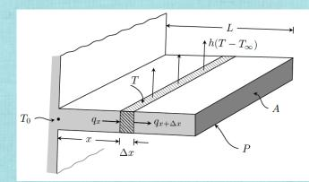
Heat in at x by conduction = Heat out by conduction at  $(x + \Delta x)$ + Heat out by convection
